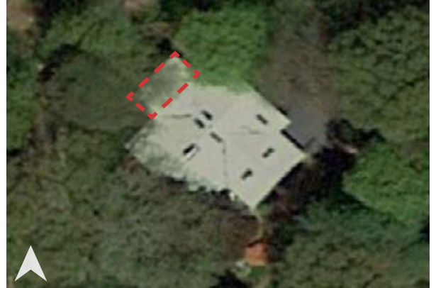
Aerial image of a house with a rear addition that is set back from the side elevations which often helps reduce visibility and differentiate an addition from the original volume (recommended) (Google Earth, 2018).
