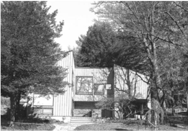
New construction with incompatible massing, roofline, and fenestration pattern (not recommended).
