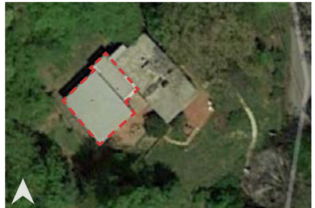
Aerial image of a house with a large two-story addition to the side elevation connected to the original building volume by a one-story hyphen (recommended) (Google Earth, 2018).
